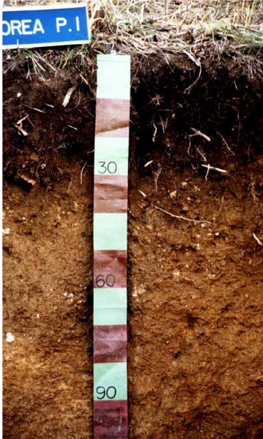
Profile of a Humudept in South Korea. This soil has an umbric epipedon about 30 cm thick. Below this epipedon is a cambic horizon that extends beyond the base of the photo. Scale colors are in 10-cm increments.
