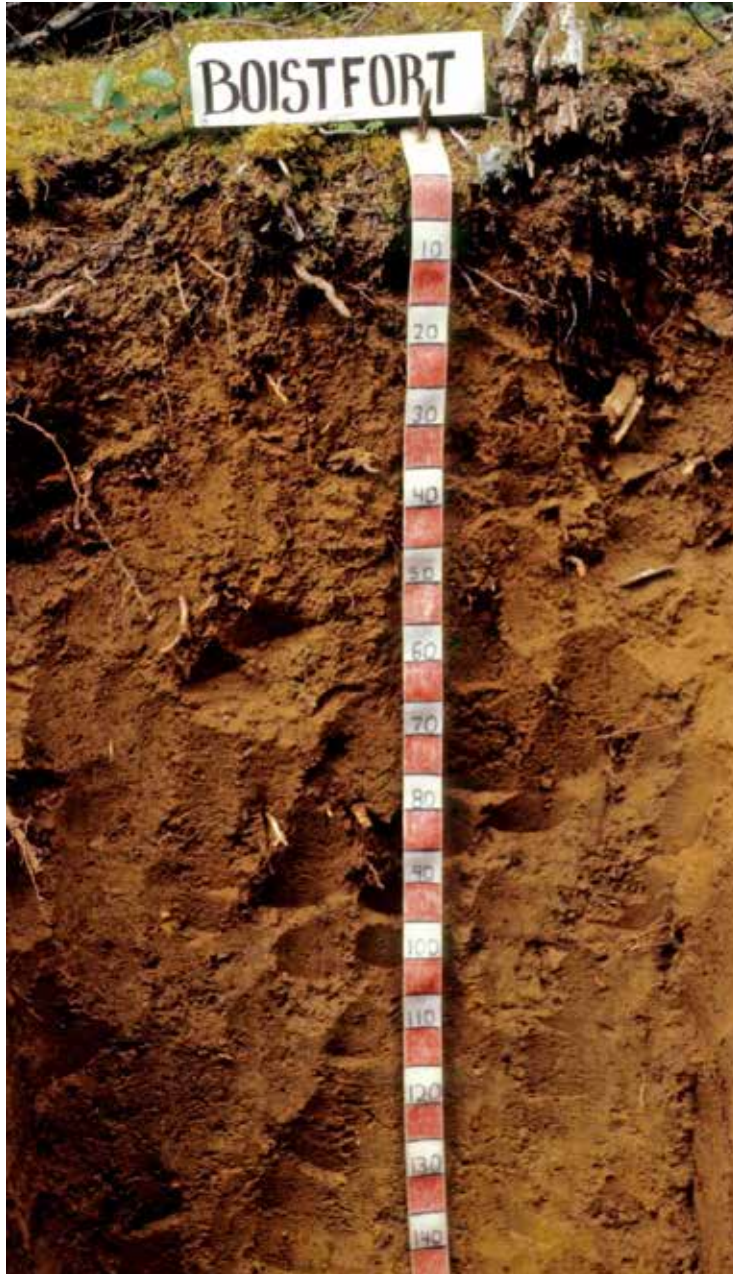
Profile of a Fulvudand in Washington State. This soil formed in material weathered from basalt bedrock with an admixture of volcanic ash in roughly the upper 50 cm. This profile has an umbric epipedon extending from the surface to a depth of about 25 cm. Below this epipedon is a cambic horizon that extends to about 120 cm. Scale is in cm.
