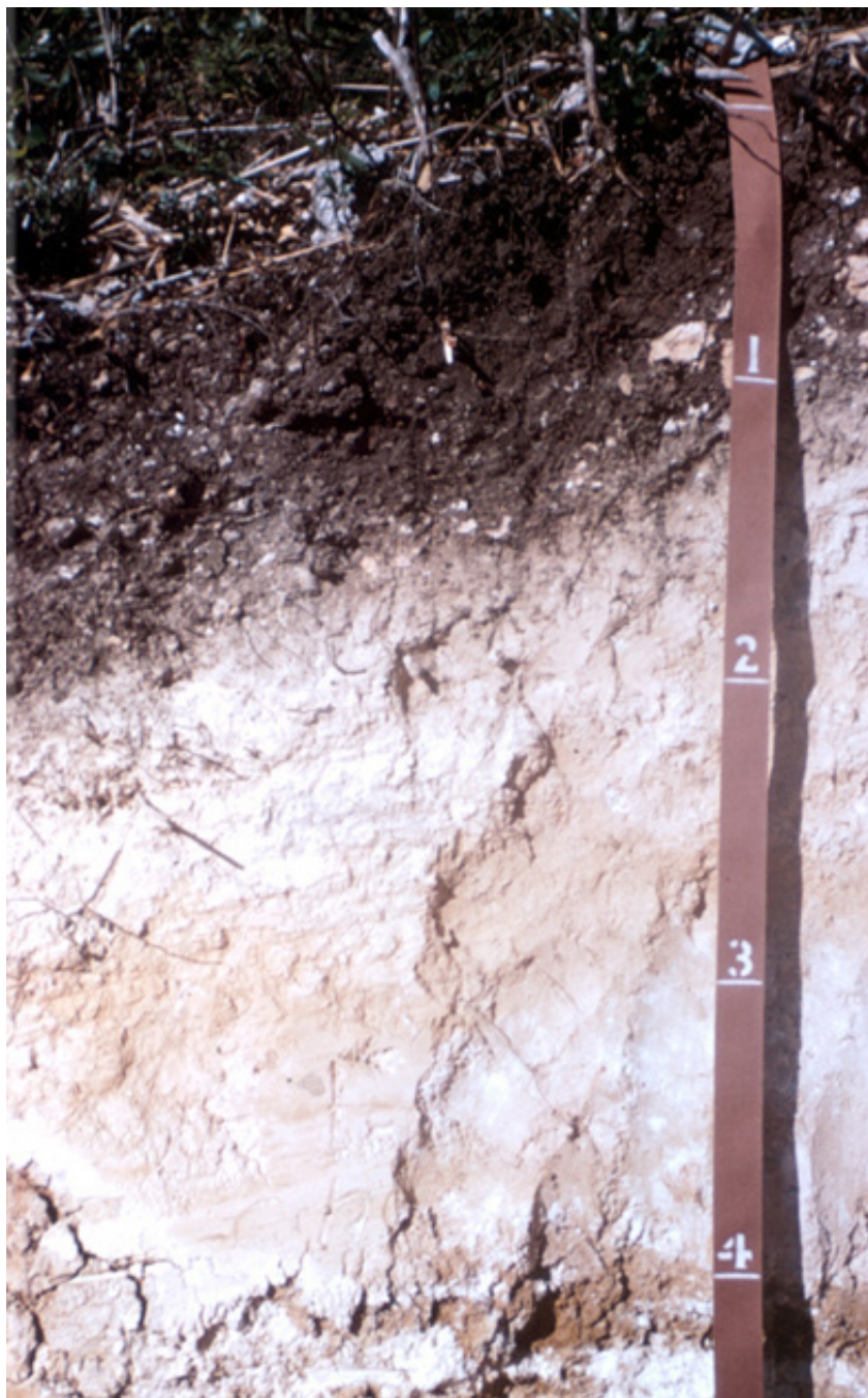
Profile of a Rendoll (specifically a Haprendoll). The mollic epipedon rests on chalk (white). Scale is in feet.
