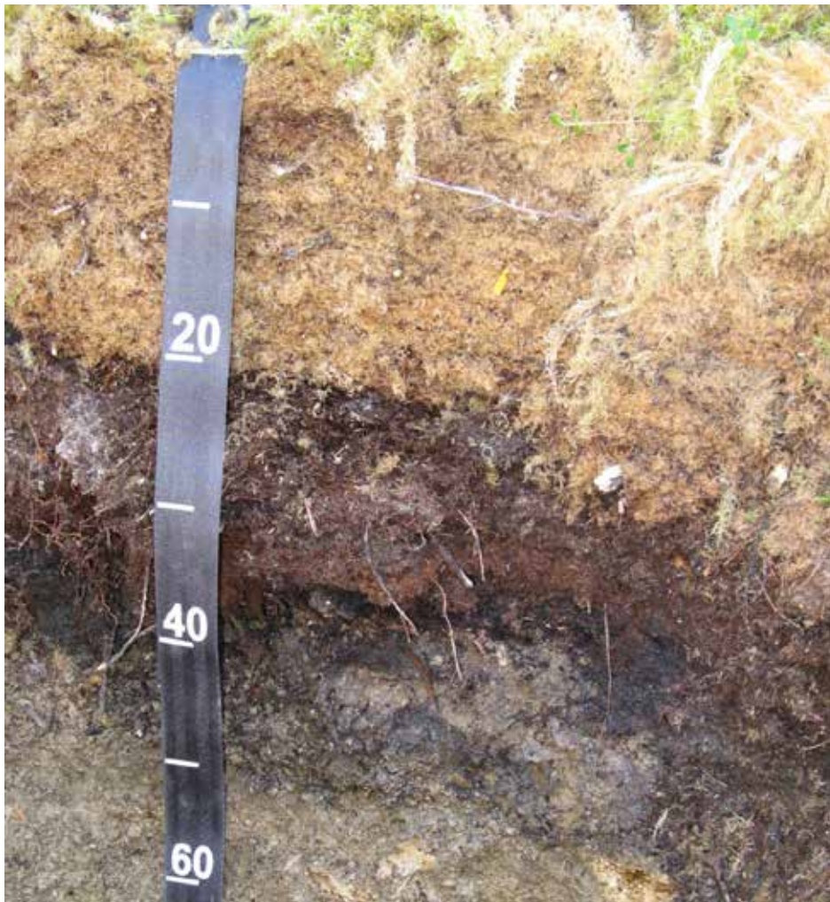
Soil profile (in Alaska) that has a histic epipedon extending to a depth of about 38 cm. The upper 20 cm is fibric soil material that has a high content of sphagnum. Scale is in cm. (Photo courtesy of Dr. David Weindorf)
