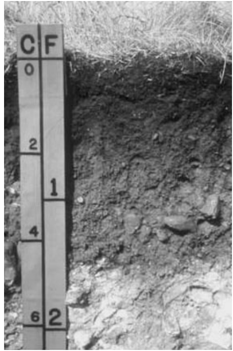
Figure 15.1. Profile photo of a Mollisol (Cryoll) from Montana showing black soil colors in the top 20 cm. Average organic matter content in the top 20 cm is approximately 6.8%. Scale is in decimeters (C) and feet (F).
