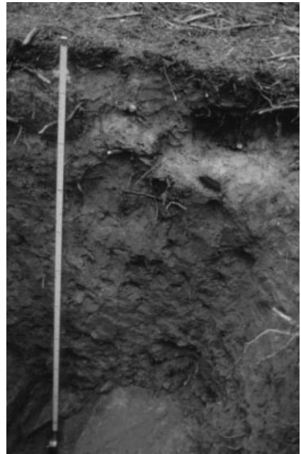
Figure 17.2. A Haplorthod in the boreal forest of southwest Sweden formed in loess over gneissic till. The pedon is about 1 m deep. For color detail, please see color plate section.
