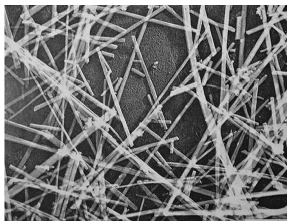
FIGURE 21.23 Electron micrograph of palygorskite from Nawton, near Thirsk, Yorkshire. (From Gard, J.A. (ed.). 1971. The electron-optical investigation of clays. Monograph No 3. Mineralogical Society, London, U.K. Reproduced with kind permission of The Mineralogical Society of Great Britain and Ireland.)
