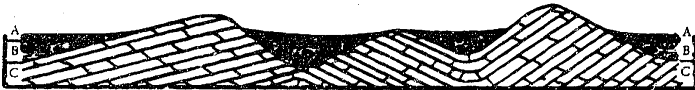
FIGURE 8. A. Soils; B. Weathering products of bedrock, often containing undecomposed fragments of the latter; C. Bedded clays, limestones, sandstones.
