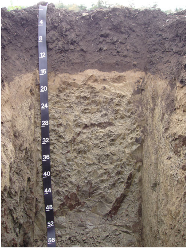
Fig. 5.2 Many soils of the Puget Sound Valley, such as this Argialboll, formed in loamy glacial deposits over compact, clayey glaciomarine sediments. The change in particle size distribution with depth results in perched water over the dense layers (image by Toby Rodgers, NRCS; NRCS file photograph released to the public domain)
