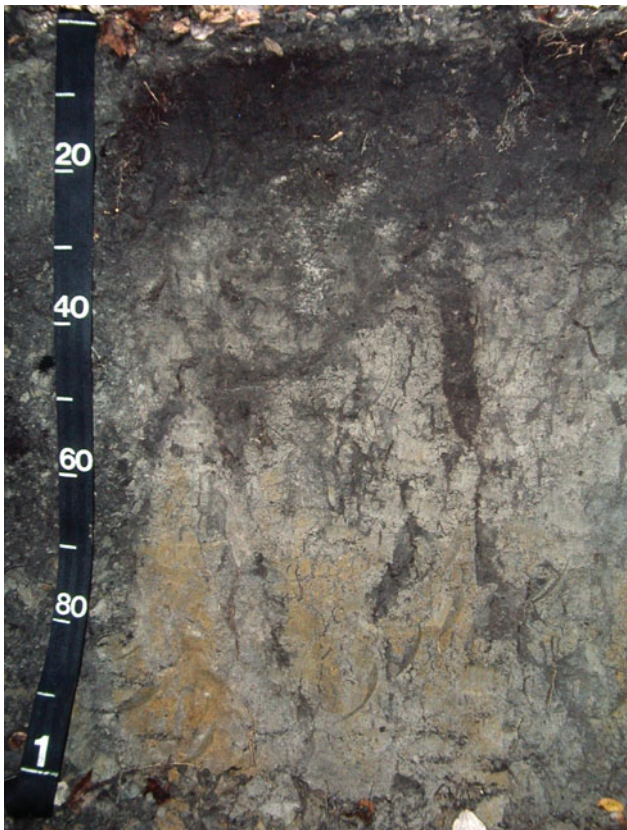
Fig. 2.7 An Ultisol with an aquic soil moisture regime (Paxville series) formed in a poorly drained depression on a broad interstream divide on the middle Coastal Plain of North Carolina. The 43–120 cm depth is an argillic horizon with gray redox depletions and yellow–red redox concentrations. The A horizon (above the 27 cm depth) is darkened by humified organic matter. Photograph credit: R.C. Graham
