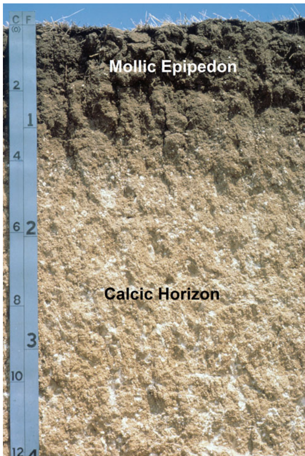
Fig. 3.2 This soil profile from a semiarid grassland area of Texas has a mollic epipedon extending from the surface to about 38 cm and a calcic horizon in the subsoil below. The dark color of the mollic epipedon is due to the relatively high content of organic matter. The white concentrations scattered throughout the calcic horizon are accumulations of calcium carbonate (scale, decimeters left , feet right ). Photograph courtesy USDA-NRCS Soil Survey Staff
