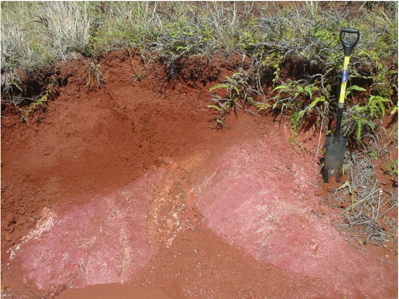
Fig. 16.14 Profile of a highly eroded Akina series (Inceptic Haplustox) developed in volcanic parent materials in Southern Guam. The pinkish colored material to the left of the shovel is dense saprolite. The
