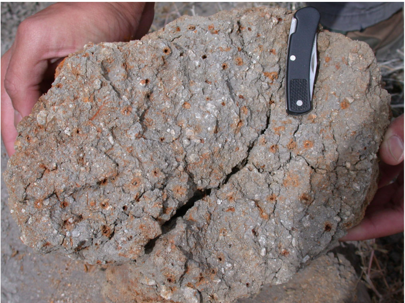
Fig. 2.12 Intact subsoil material from a soil formed in a wetland in Owens Valley, California. The gray matrix was depleted of iron oxides by reducing conditions, while iron oxides precipitated around the oxygenated root channel macropores
