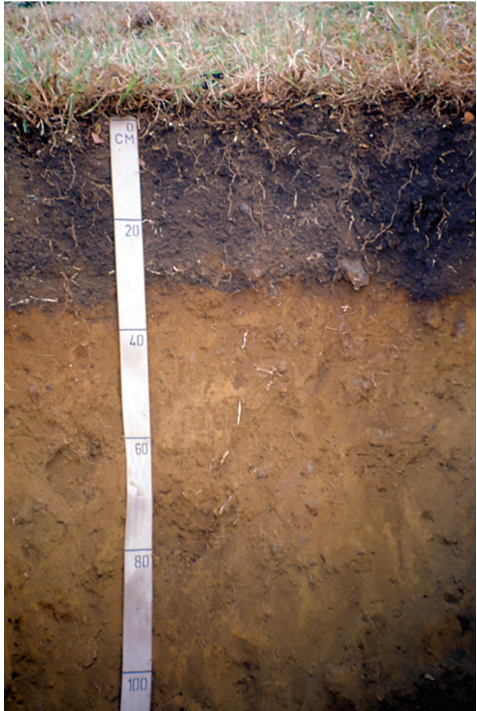
Fig. 16.5 Profile of the Kealakekua series (Typic Hydrudands), a moderately deep, hydrous Andisol found on the Big Island of Hawaii
