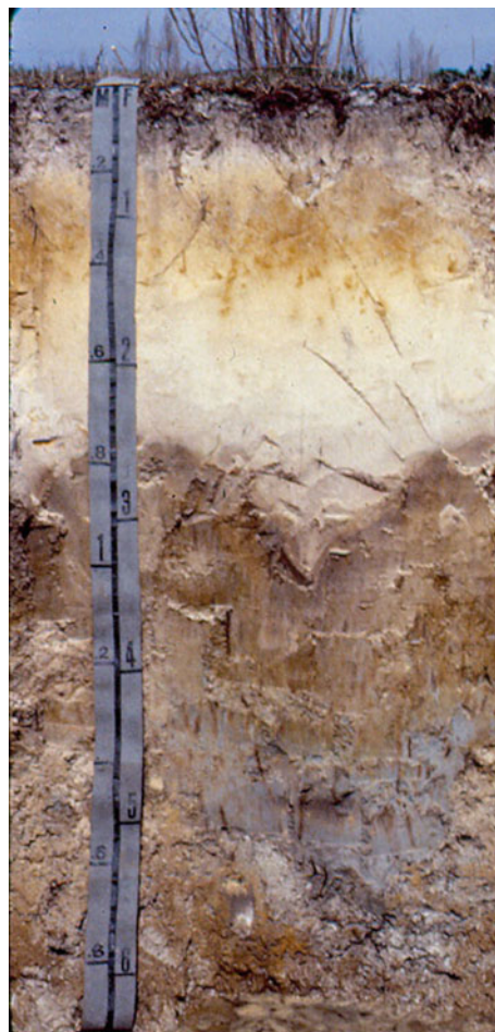
Fig. 15.16 Pineda series in MLRA 155—Southern Florida Flatwoods. These poorly drained soils formed in thick deposits of sandy and loamy marine sediments and occur on broad low flats, hammocks, sloughs, depressions, and poorly defined drainageways and flood plains
