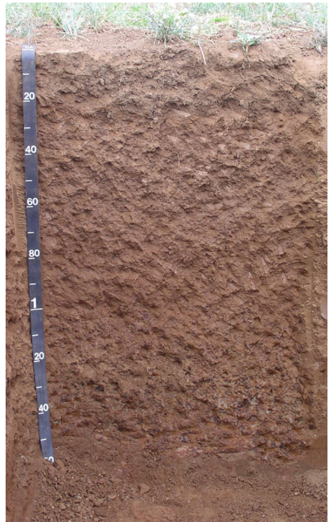
Fig. 5.3 Jory, a Palehumult, is the state soil of Oregon. It is well-drained, very deep, and formed in clayey colluvium derived from mafic igneous rock. The soil temperature regime is mesic and the moisture regime is xeric. Depths are in cm (NRCS file photograph released to the public domain)
