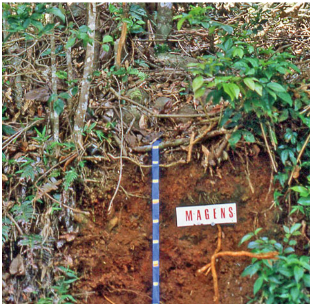
Fig. 15.32 Magens soil series in MLRA 271—Semi-arid Mountains and Valleys (Virgin Islands). The soils are very deep, well drained, medium to strongly acid, moderately permeable
