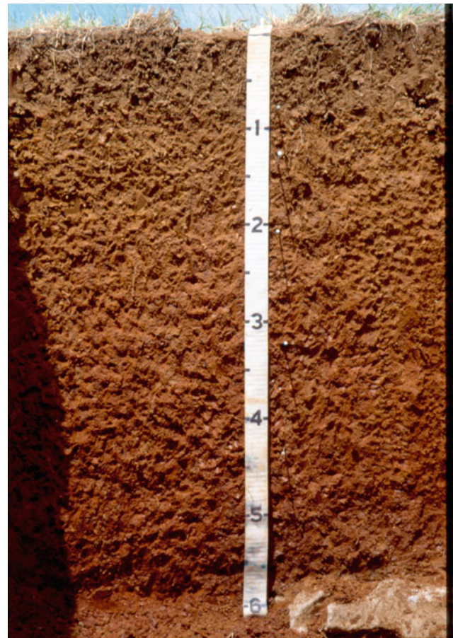
Fig. 12.9 Paleudalf (Crider series, State soil of Kentucky) is a well-drained soil formed from limestone residuum found in upland landscape positions of the Pennyroyal Plateau. Photograph credit Jerry McIntosh
