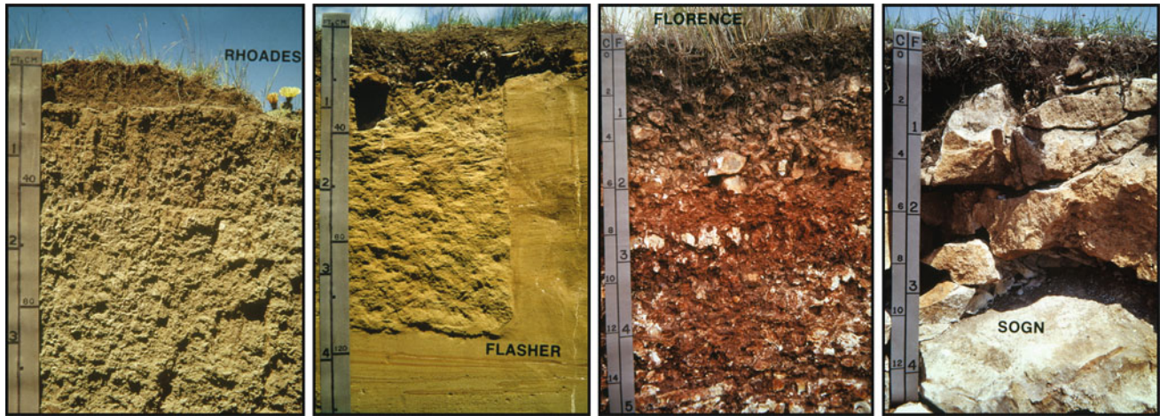
Fig. 8.19 Several soil profiles developed in bedrock residuum. The very slowly permeable Rhoades series (Leptic Vertic Natrustolls) formed in soft shale, siltstone, and mudstone in upland swales. By contrast, the Flasher series (Typic Ustipsamments) is excessively drained with a moderately rapid to rapid permeability and developed from soft sandstone within the same MLRA (54). Similarly, the
