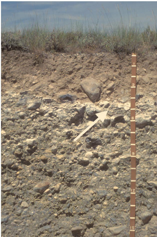
Fig. 6.2 Relatively light-colored A horizon and thin SiO 2 - and CaCO 3 -cemented duripan (arrow) in a very gravelly Haplodurid. Cementation occurs between approximately 40 and 55 cm. Scale is in decimeters
