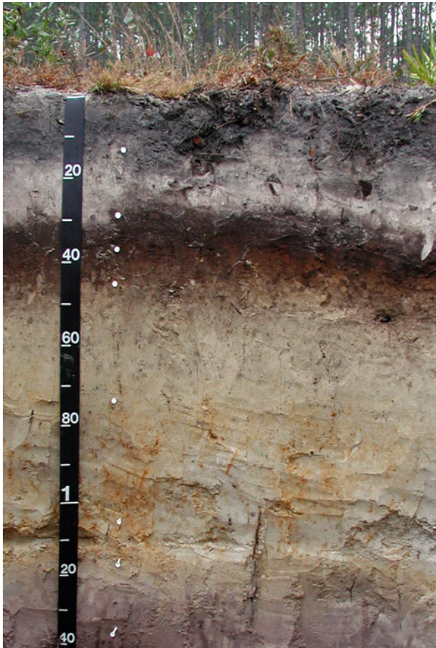
Fig. 13.11 Typical Alaquod from MLRA 153A. The Bh horizons (spodic horizons) underlie an albic E horizon at 30 cm and extend to about 45 cm. Underlying the Bh horizons are E' horizons that extend to about 125 cm. A second spodic horizon (B'h horizon) underlies the E' horizons. Photo credit: LT West
