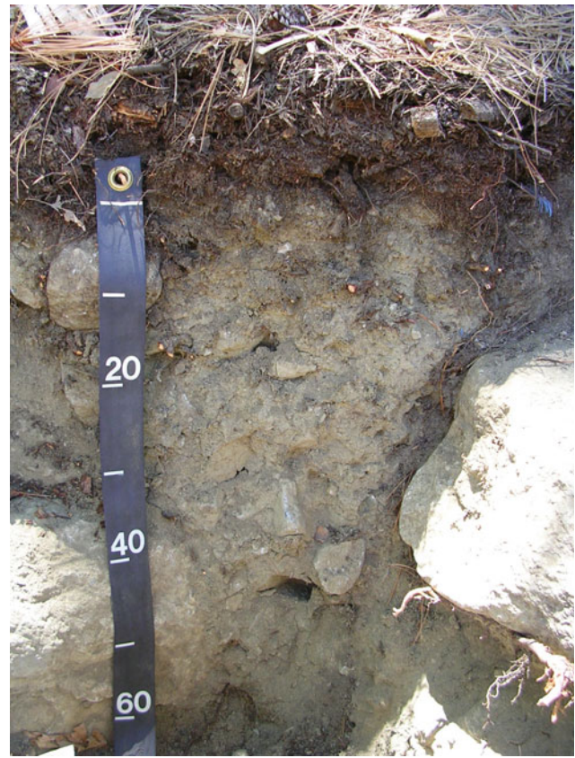
Fig. 2.2 An Entisol formed in a debris flow deposit in the San Bernardino Mountains, California. The pine needles, twigs, and other plant parts that compose the O horizon at the surface become more decomposed with depth. Photograph credit: Judith Turk
