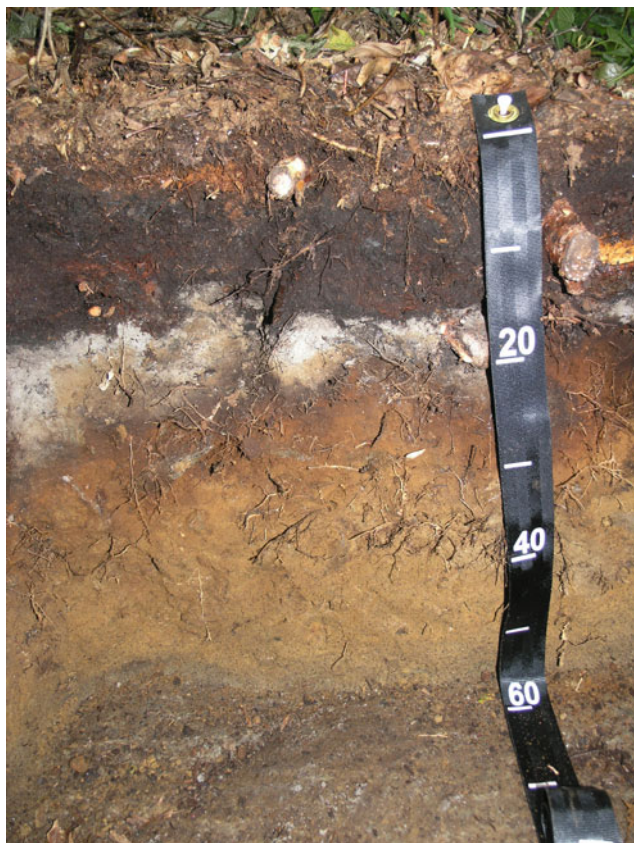
Fig. 14.12 Profile of a Lithic Haplorthod in MLRA 144B. The profile has 18 cm of O horizon (Oi and Oa), an albic E horizon, Bhs horizon, and Bs horizon. The contact with the R horizon is at 62 cm
