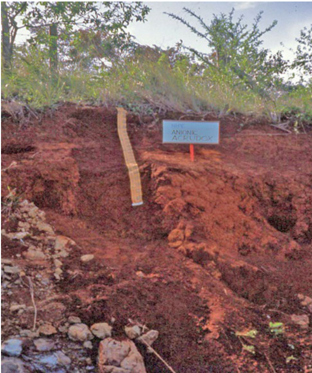
Fig. 15.29 Nipe soil series in MLRA 270—Humid Mountains and Valleys (Puerto Rico). These soils are very deep, moderately to strongly acid, moderately permeable on ridge tops of hills and mountains (2–20 % slopes). The parent material is iron-rich residuum which weathered from serpentine bedrock
