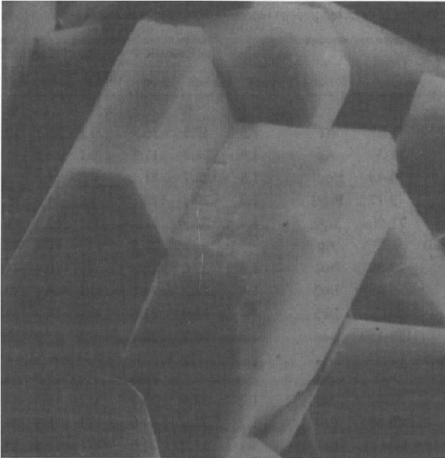
FIGURE 33.83 Scanning electron micrograph of a gibbsite nodule in a Gibbsiudox from Malaysia; the gibbsite crystals are typically euhedral and fine and medium silt size; magnification \times 10,000 .
