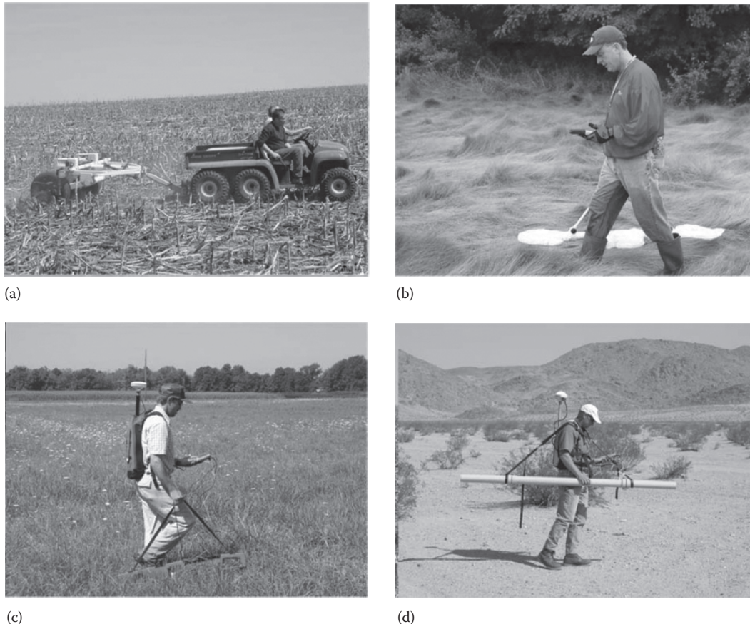
FIGURE 39.12 Selected EMI equipment. Pictured are the Veris Soil EC 3100 mapping system (a); the Profiler EMP-400 multifrequency sensor (b); the EM38 meter (c); and the Dualem-2 meter (d).
