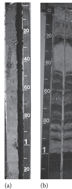
FIGURE 36.4 (a) Vibracore profile of a Haplic Sulfiwassent from a shallow mainland cove. The tape shows 10 cm increments. Note the clam krotovina from 30 to 50 cm (C/A horizon). The white pieces in the krotovina are shell fragments. At 120 cm, there is a change in parent material from the Holocene aged estuarine sediments to the Pleistocene outwash sand and gravels. (b) Vibracore profile of a Sulfic Fluviwassent. The soil was collected from a washover-fan slope. Note the many buried A horizons that represent storm surges. The buried A horizon starting at a meter represents the upper part of a previous Typic Sulfiwassent prior to encroachment of the washover fan over the lagoon bottom landscape unit.
