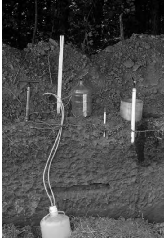
FIGURE 5.17 Photograph showing an installed tension-free pan lysimeter. Directly above the right corner of the pan is a suction cup lysimeter (diagrammed in Figure 5.20). The berm contains the excavated soil that will be returned to the soil pit after pan installation. (Photograph courtesy of Dr. Donald Tyler, West Tennessee Experiment Station, The University of Tennessee.)
