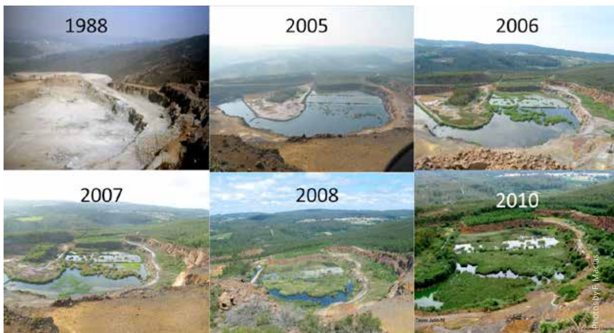
Figure 4.9 | Use of different Technosols derived from wastes in the recovery of hyperacid soils and waters in the restored mine of Touro (Galicia, NW Spain).
