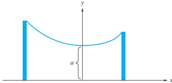
Figura 4.36 Cable suspendido
