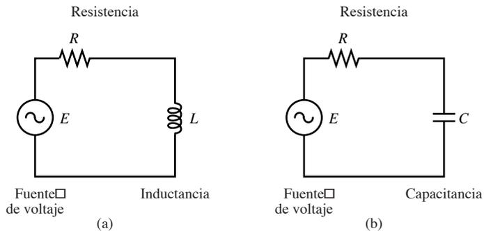
**Figura 3.13** (a) Circuito  $RL$  y (b) circuito  $RC$
