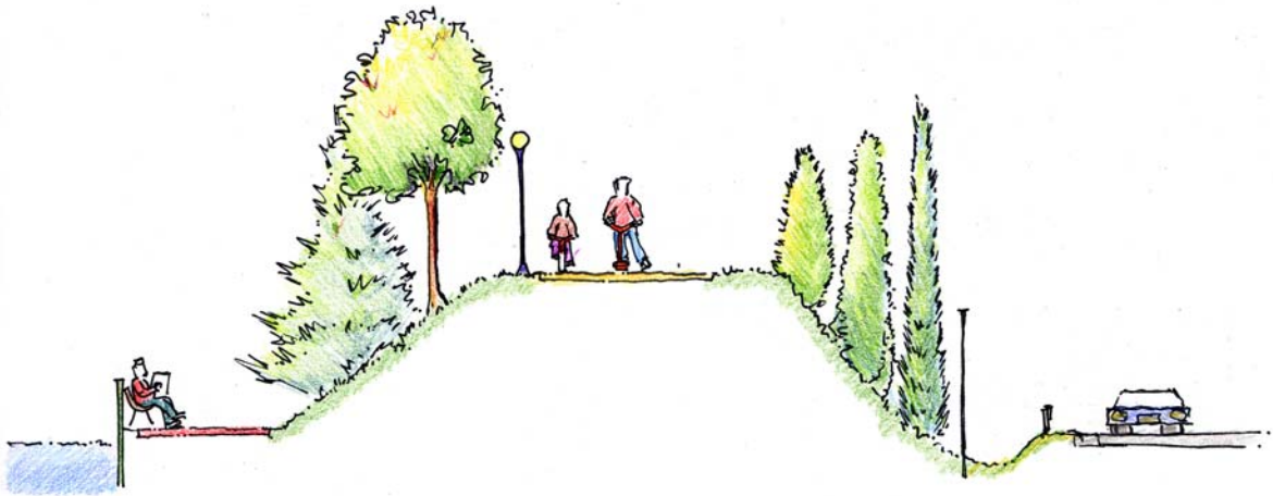
Sketch showing the use of dense planted conifers on a slope as an effective barrier against traffic noise and pollution. Scattered hardwoods allow for park views on the other side.
