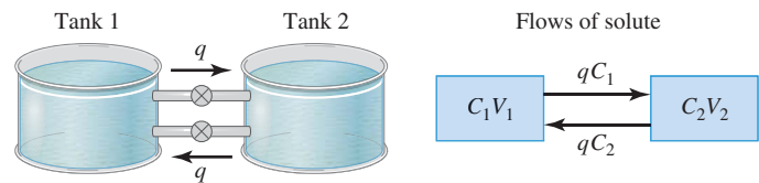
Figure 8.59 Schematic of two-compartment model for Problem 29.
