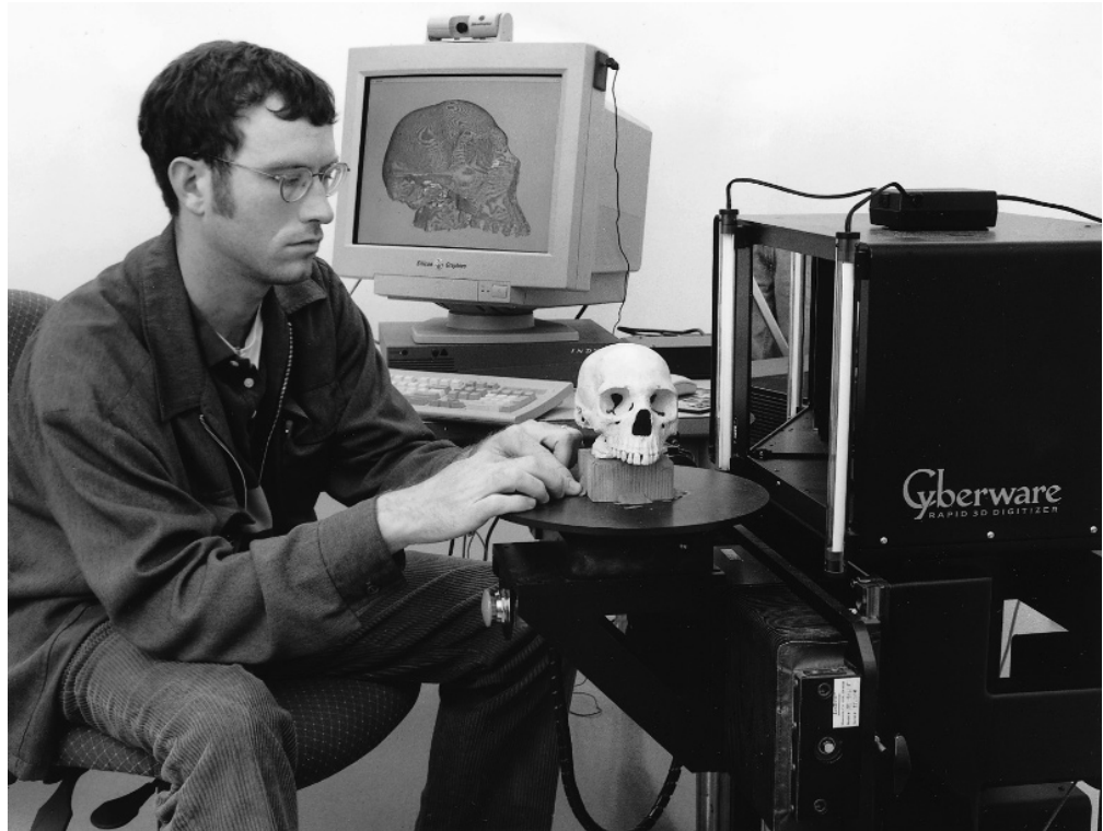
Figure 16.6 A three-dimensional laser-scanning unit at the University of California, Berkeley. The machine accurately measures three-dimensional surface topography and sends these data to a computer where measurements, restorations, and other manipulations are possible.
