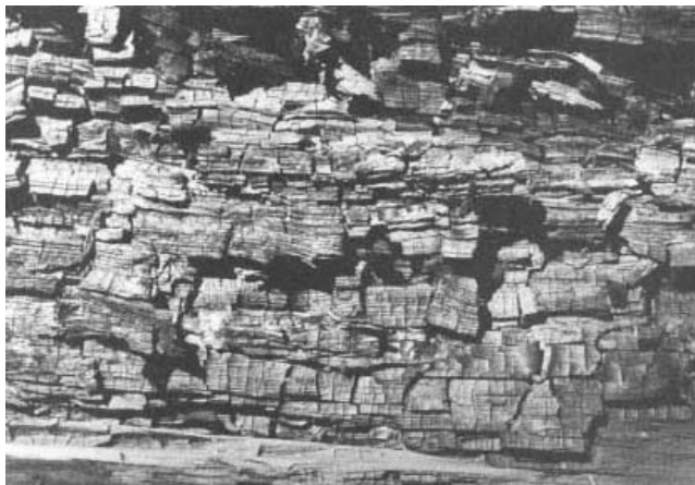
Fig. 7.8. Severe brown rot on log bench, Cortez, Colorado.
