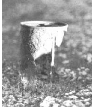
Fig. 2.1. The corroded remains of a steel can repose on the surface, Valle de la Luna, northern Chile.
