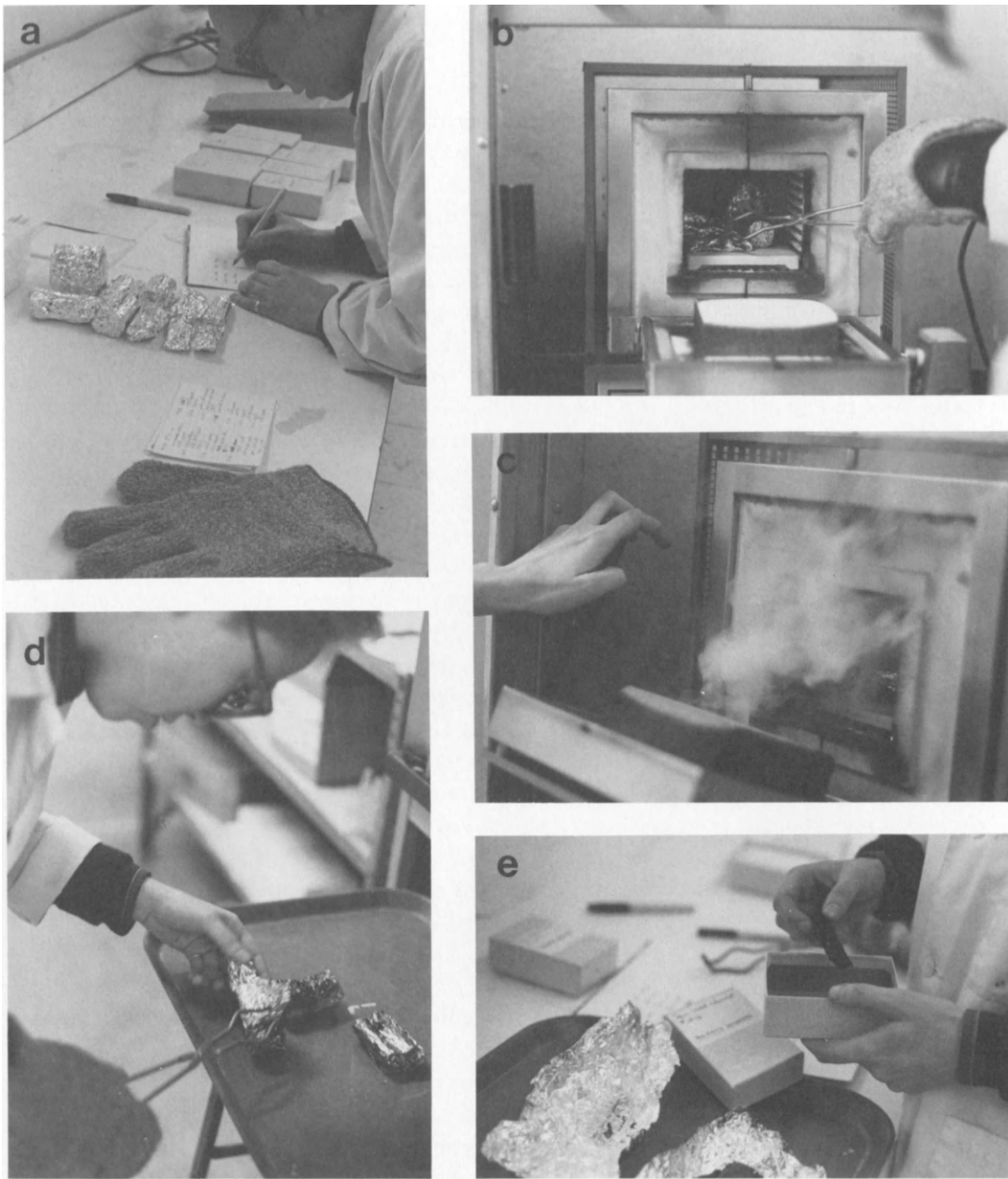
Figure 3.13 Charring comparative wood specimens in a muffle furnace: (a) specimens are wrapped in aluminum foil labeled with specimen numbers; (b) specimens are stacked in the preheated furnace, and a diagram of the arrangement of specimens is made; (c) specimens are heated until smoke no longer escapes from the furnace; (d) specimens are unwrapped and allowed to cool completely; (e) charred wood is stored in boxes in the comparative collection.
