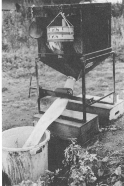
Figure 2.8 The froth flotation devise used by Crawford to recover botanical materials from Jomon period sites in Japan (photograph by G. Crawford).
