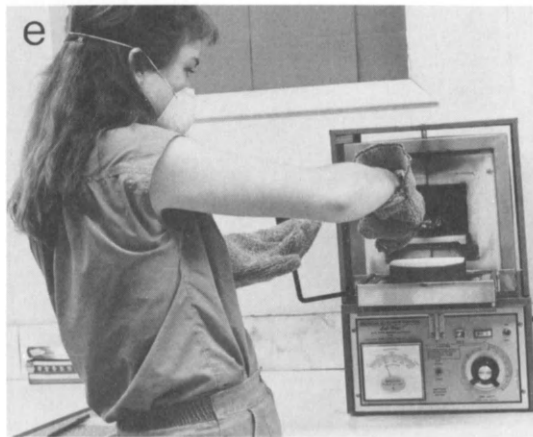
Figure 5.21 Dry ashing comparative material: (a) material for each sample is selected and placed in a beaker; (b) material is washed with distilled water to remove surface dust and other debris; (c) washed material is placed in aluminum ashing boats; (d) material is dried in a low-temperature oven; (e) dried material is transferred to a muffle furnace and heated at 400–500°C for several hours; (f) samples are finished when residue is a whitish-gray color.
