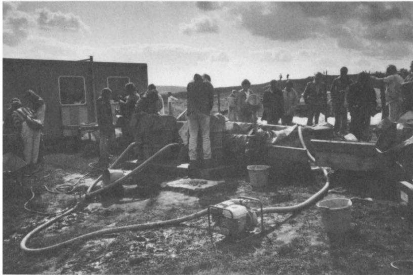
Figure 2.24 Recycling water for flotation using a settling tank system, Maiden Castle, Dorset, England. Two flotation machines are set up to run from a single two-stage settling tank system.
