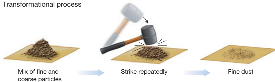
FIGURE 2.19 Different processes of change. In a transformational process, the ensemble changes because each individual member changes. In a variational process, the ensemble changes because something sorts among the variants in the original ensemble. In this example, crushing the soil particles is a transformational process—the ensemble shifts toward smaller particles because the individual particles are reduced. Sifting the soil is a variational process—the ensemble shifts toward smaller particles because the larger particles are sorted out.
