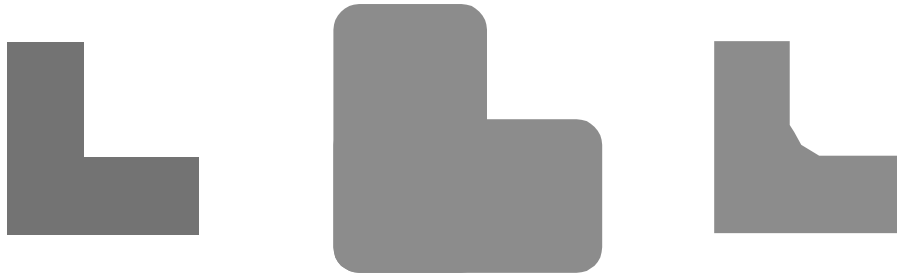
Figure 6: The 2D shape (left) may be filleted (right) by first expanding it via a Minkowski sum with a disk of radius r (center) and then by shrinking the result via a Minkowski difference with the same disk. Subtracting the original shape from the filleted version yields solid fillets that may be easily trimmed before being added to the original solid.
