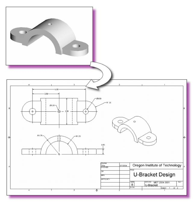
The 2D drawing is generated from the 3D model. Any modifications made to the 3D model at any time are automatically reflected on the 2D drawing.
