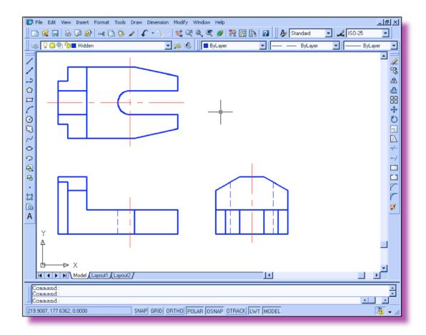
Note that (1) the creation of these views requires knowing the dimensions and (2) each of the three views is created and edited independently of the others, as shown in the figure below. Changes in one view are not automatically reflected in the other views. Each view has to be updated manually.
