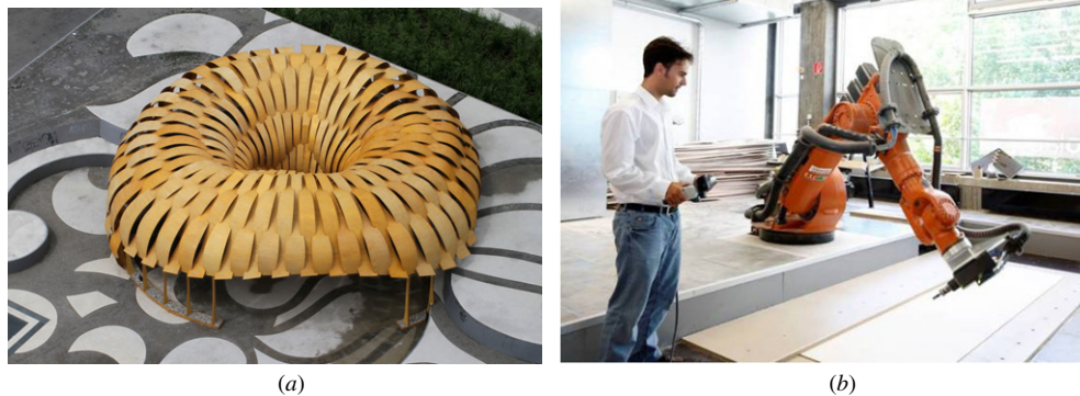
Figure 3. (a) ICD/ITKE Research Pavilion 2010, University of Stuttgart (photo: Roland Halbe), (b) digital fabrication of plywood strips (photo: University of Stuttgart).
