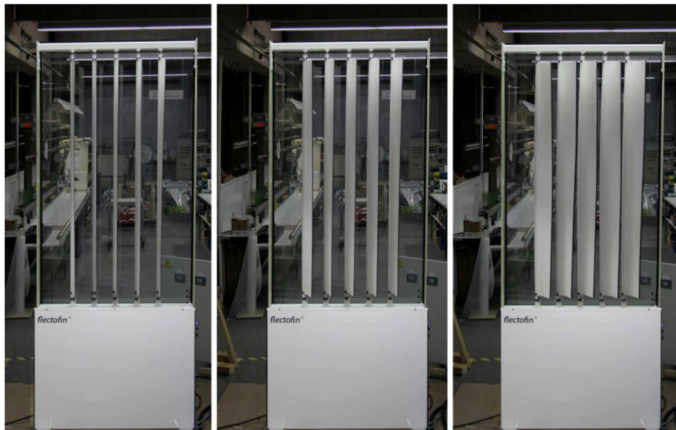
Figure 8. Prototype of the façade shading system based on the Flectofin ® produced in collaboration with the industrial partner Claus Markisen (adapted from Lienhard et al 2011b).
