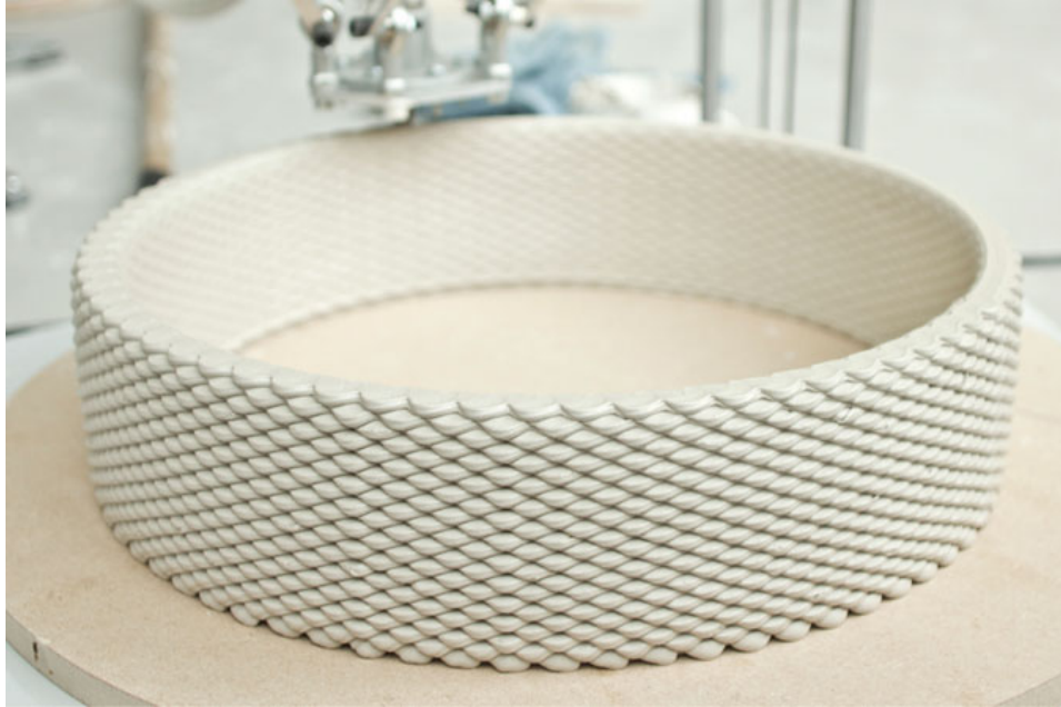
88 . 3D-printed ceramic by Olivier van Herpt showing the beauty and precision with which relatively crude materials like mud and clay can be assembled
