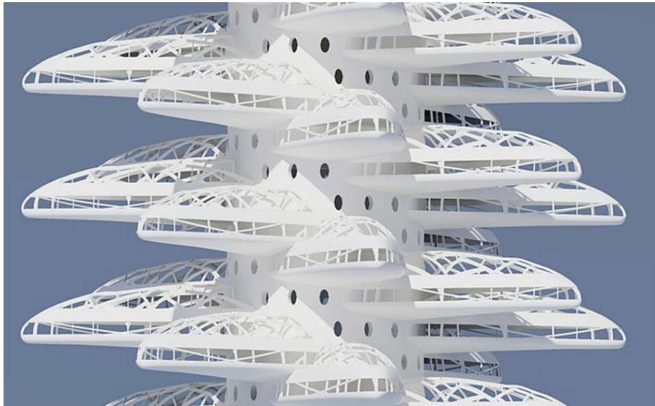
129 . Phyllotactic tower by Saleh Masoumi, based on the geometry of plants, which optimises access to light by minimising self-shading between leaves
