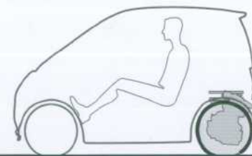
Rear Transverse Engine - RWD
