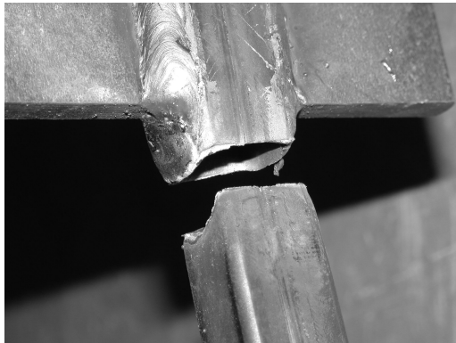
Figure 8. Typical failure of 20x20x2.0SHS long specimen (Series 3)
