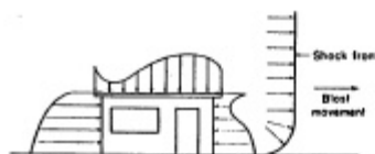
Fig. 5. Blast load on a fully engulfed building.
