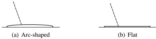
Fig. 4. Examples of feet. As long as the toe and heel are the only contact points with the ground, (a) and (b) are equivalent.
