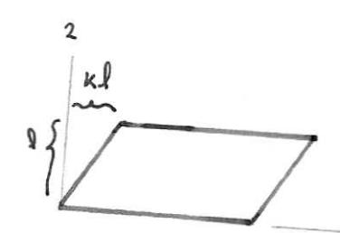
$$\Rightarrow [\underline{\underline{B}}] = [\underline{\underline{E}}][\underline{\underline{F}}]^T = \begin{pmatrix} 1 & k & 0 \\ 0 & 1 & 0 \\ 0 & 0 & 1 \end{pmatrix} \begin{pmatrix} 1 & 0 & 0 \\ k & 1 & 0 \\ 0 & 0 & 1 \end{pmatrix} = \begin{pmatrix} 1+k^2 & k & 0 \\ k & 1 & 0 \\ 0 & 0 & 1 \end{pmatrix}$$
