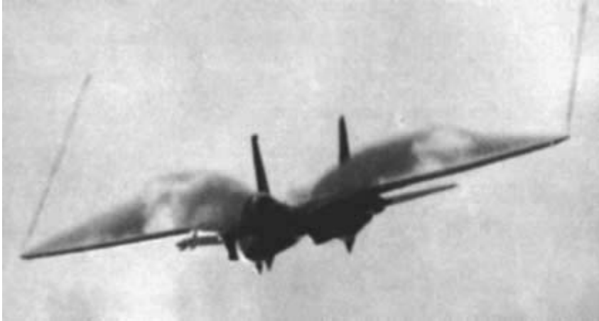
Fig. 2.19. Illustration of the lift distribution on the wings of an F-14A. (Photo courtesy of NASA.)
