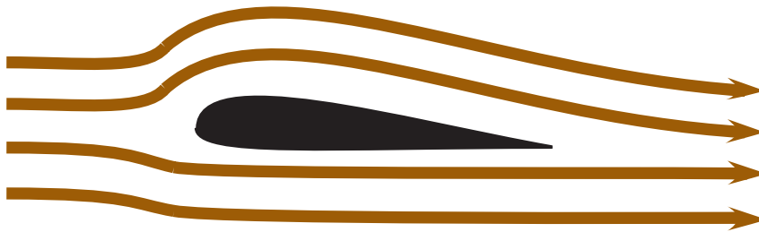
Fig. 2.2. Based on Newton's laws, this airfoil has no lift.
