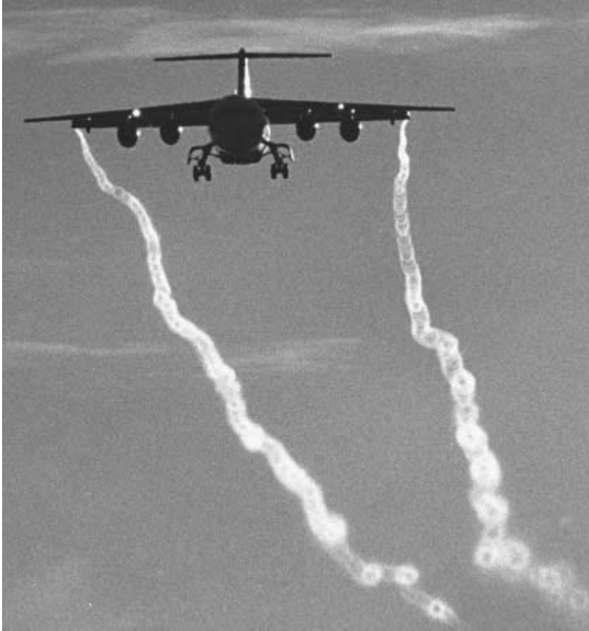
Fig. 2.21. Wing flap vortices. (Photographer, Jan-Olov Newborg.)
