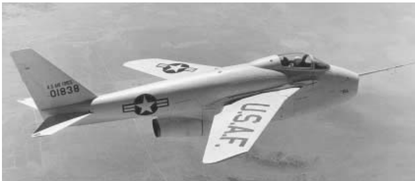
Fig. 3.7. The variable-sweep X-5 research aircraft. (Photo courtesy of NASA.)
