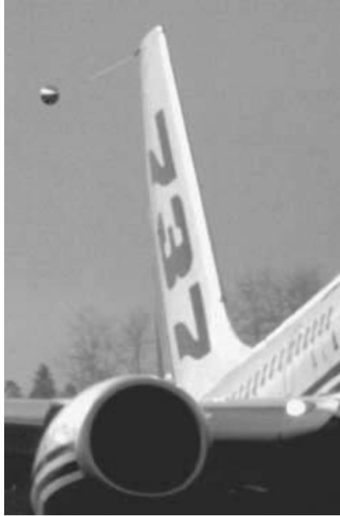
Fig. 8.21. Trailing cone on 737-700. (Used with the permission of the Boeing Management Company.)
