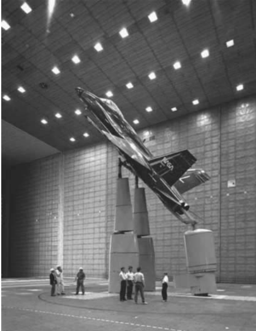
Fig. 8.11. Test section of the NASA Ames 80 \times 120 open-circuit wind tunnel. (Photo courtesy of NASA.)
