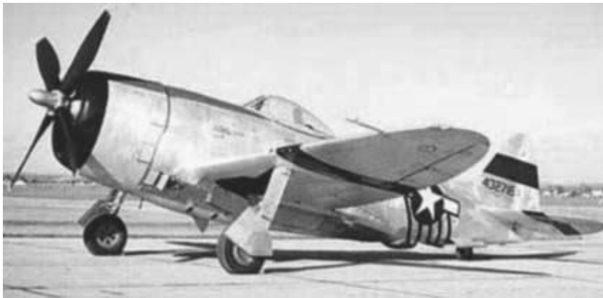
Fig. 3.12. The Republic P-47 with an elliptic wing shape. (Photo courtesy of the U.S. Air Force Museum.)
