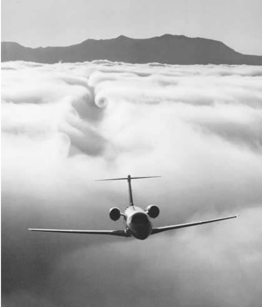
Fig. 2.7. A jet flying over fog demonstrates downwash. (Photographer Paul Bowen; photo courtesy of Cessna Aircraft Co.)
