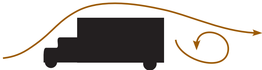
Fig. 3.23. Form drag illustrated by the wake of a truck.
