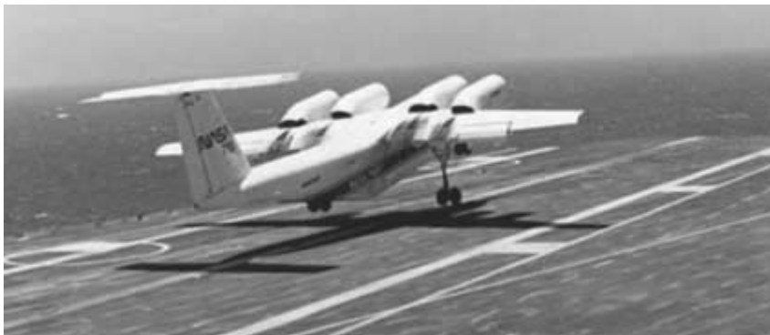
Fig. 3.34. NASA QJRA STOL research vehicle with deflected jetwash. (Photo Courtesy of NASA.)
