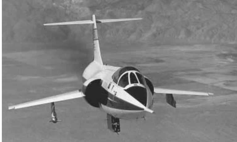
Fig. 3.15. The F-104 with anhedral (negative dihedral). (Photo courtesy of NASA.)
