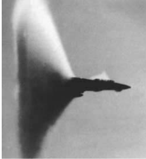
Fig. 6.1. Transonic F-18 with shock wave over wing. (Photo courtesy of the U.S. Air Force.)
