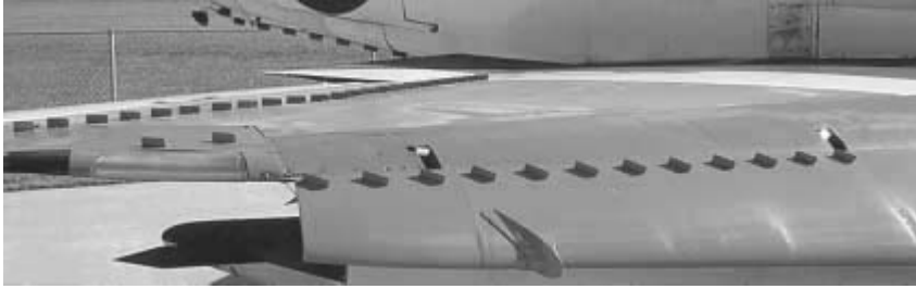
Fig. 3.25. Vortex generators on the slat and wing of a Navy A-4 Sky Hawk. (Air Classics Museum, Aurora, IL.)
