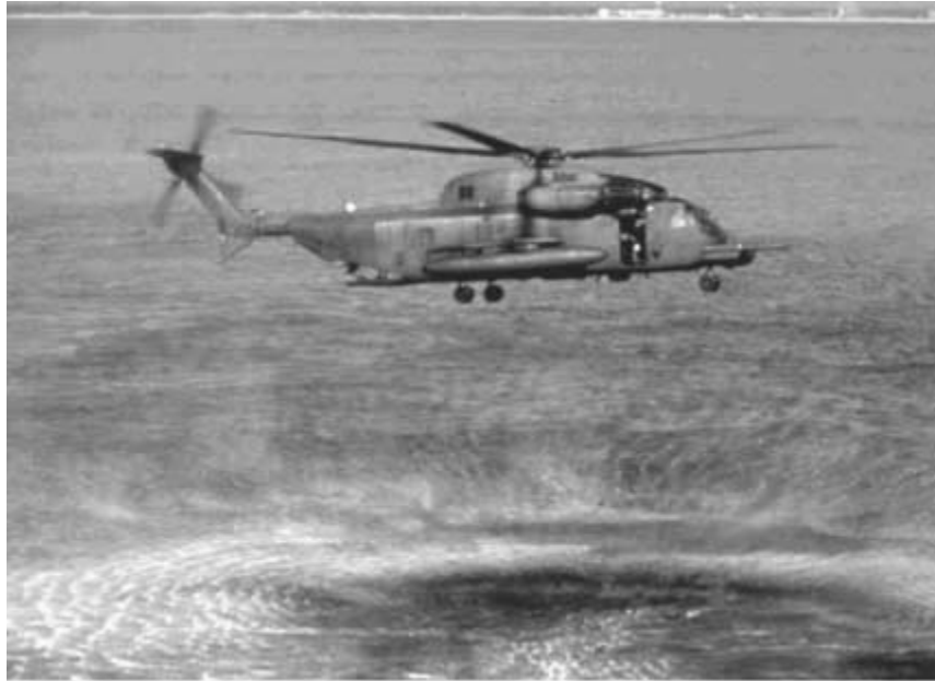
Fig. 2.8. A helicopter pushes air down. (Photo courtesy of the U.S. Air Force.)
