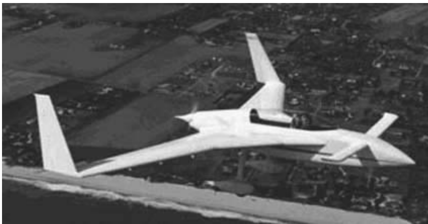
Fig. 3.19. A home-built Long-EZ illustrating a canard configuration. (Photo courtesy of Sandy DiFazio.)
