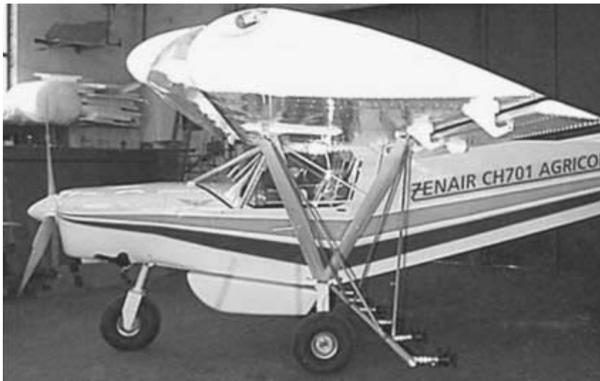
Fig. 3.4. A STOL airplane with a fat leading-edge wing. (Photo courtesy of Czech Aircraft.)
