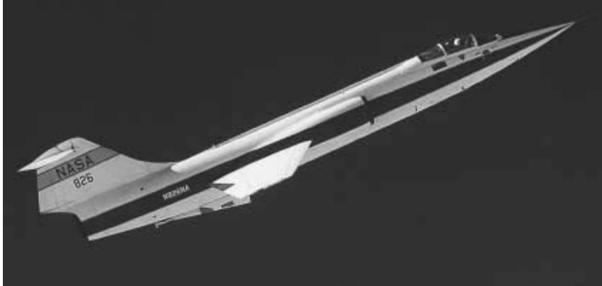
Fig. 3.3. The F-104 Star Fighter with a thin sharp wing. (Photo courtesy of NASA.)
