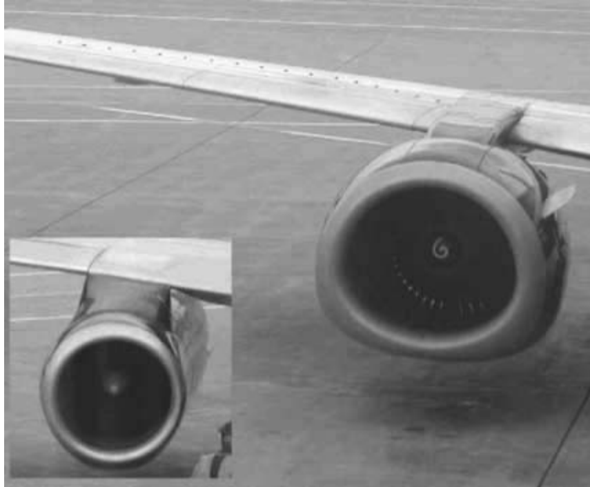
Fig. 3.17. The Boeing 737 noncircular engine inlets with the old engine as insert.
