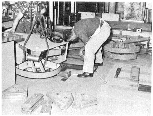
Fig. 3. Vibration Exciter Unit Being Installed in Laboratory
