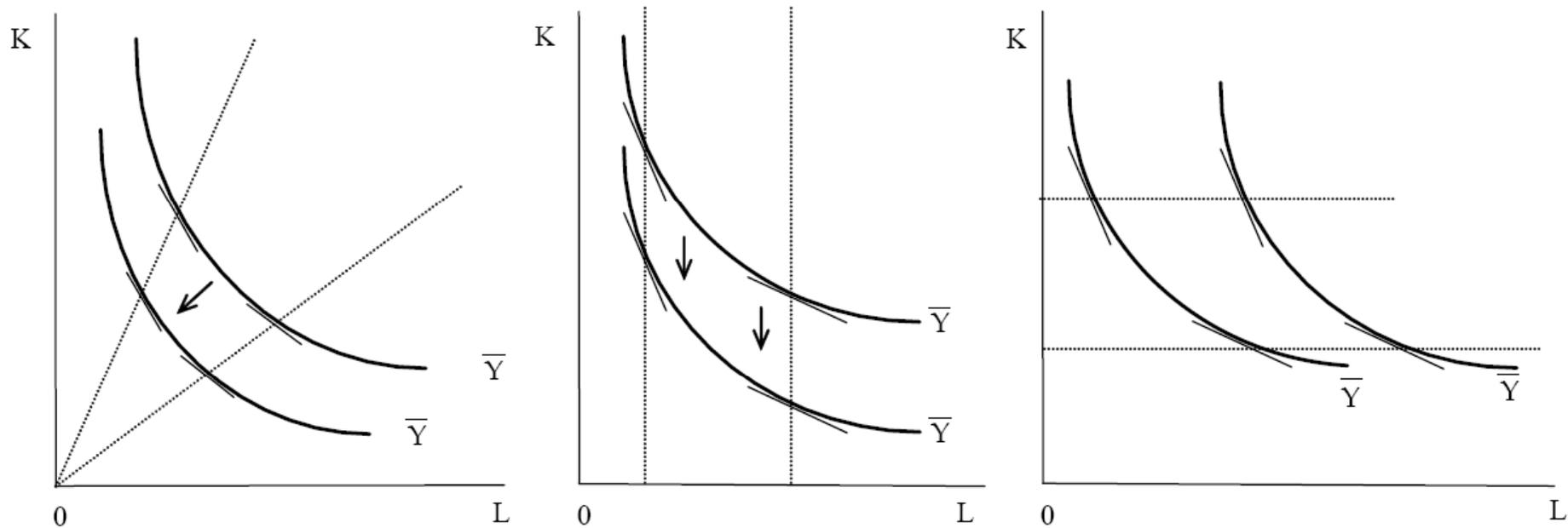
FIGURE 2.12. Hicks-neutral, Solow-neutral and Harrod-neutral shifts in isoquants.
