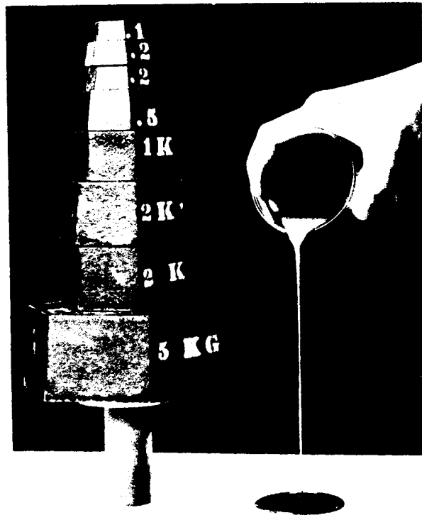
Fig. 2.9 (a) Undisturbed and (b) thoroughly remolded sample of Leda clay from Ottawa, Ontario. (Photograph courtesy of the Division of Building Research, National Research Council of Canada. Hand by D. C. MacMillan.)
