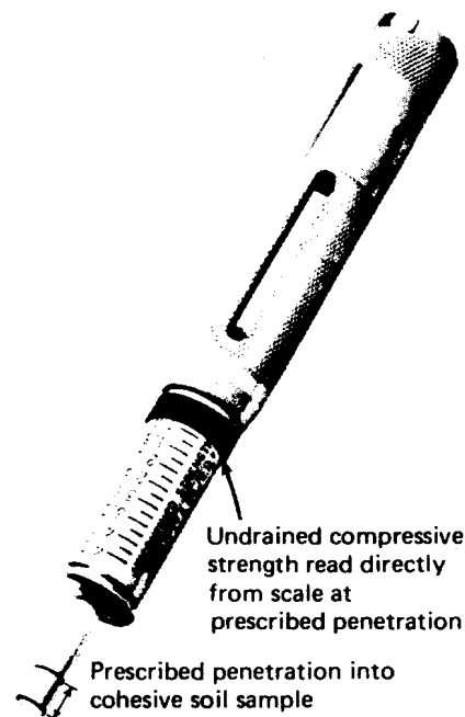
Fig. 11.47 Pocket penetrometer (PP), a hand-held device which indicates unconfined compressive strength (photograph courtesy of Soiltest, Inc., Evanston, Illinois).
