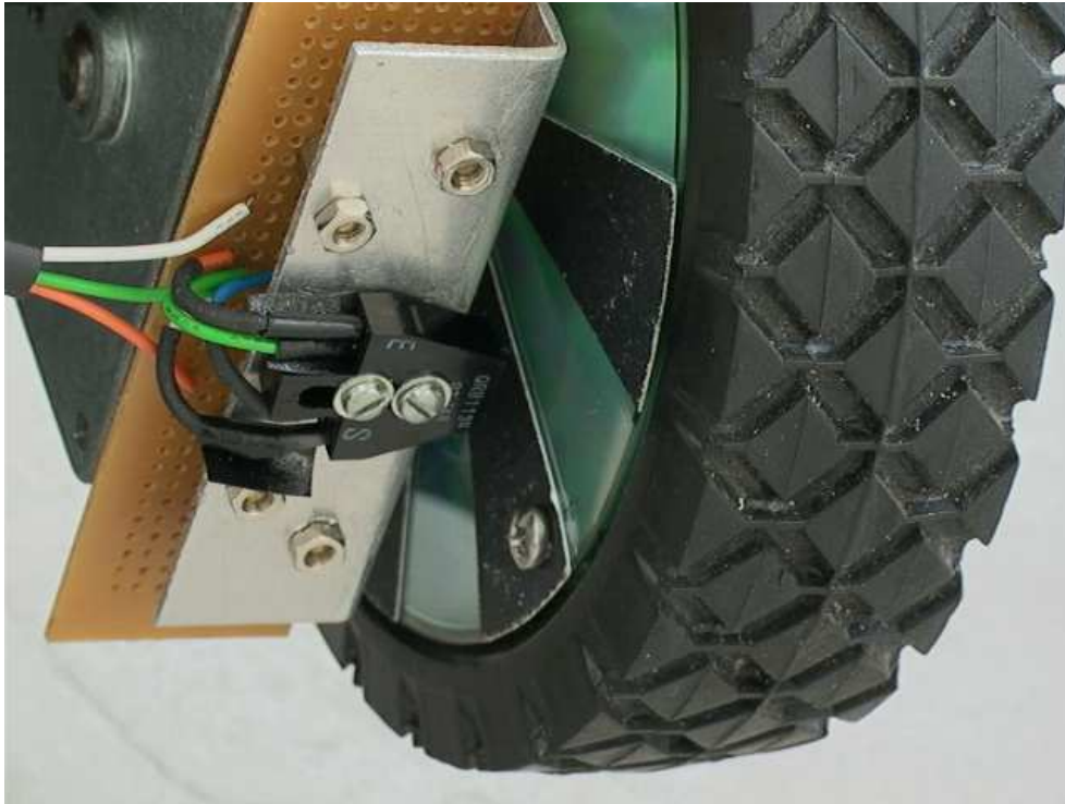
Figure 2: A photo of a wheel encoder. The reflective disc (rigidly fixed to the inside of each wheel) has non reflective (black) tape spaced evenly over its reflective area. The black plastic sensor, contains an L.E.D. and receiver photo-diode, which receives light reflected back from the L.E.D. When a reflective segment of the disc is in front of the sensor, the photo-diode output is high, but when black tape is present, the output will be low.
