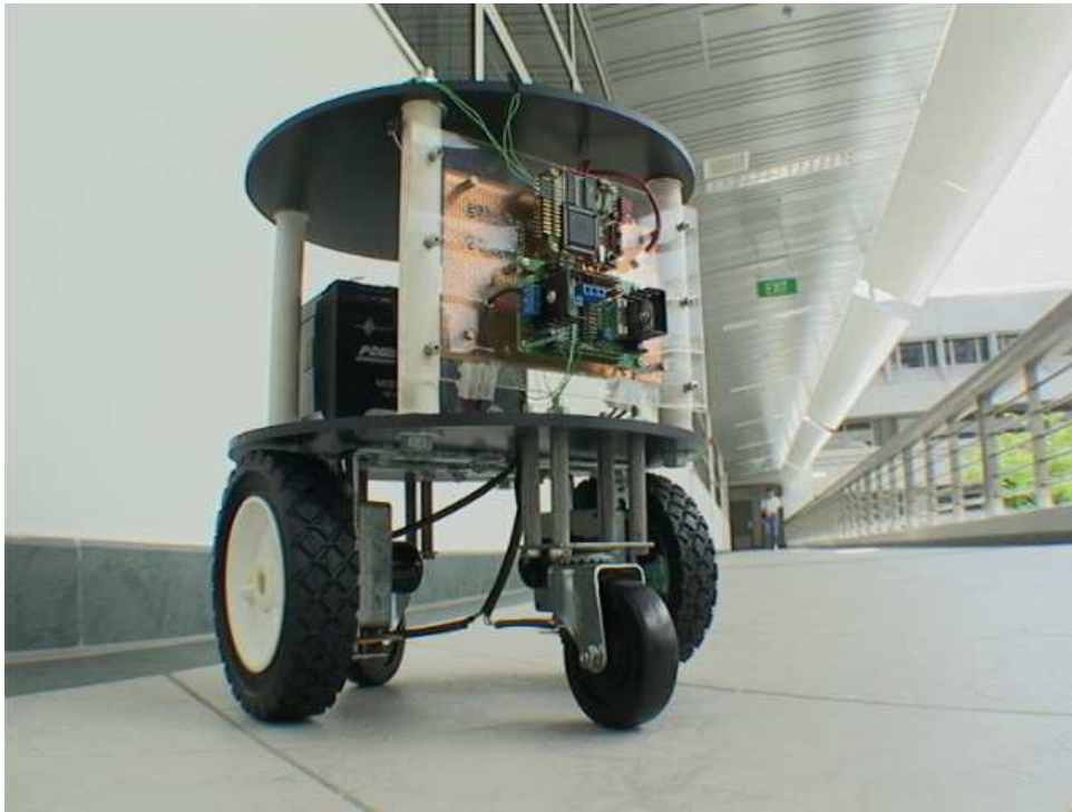
Figure 1: A photograph showing an actual, differential drive mobile robot platform.
