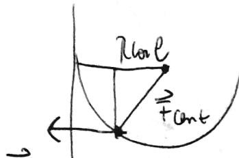
$$\begin{aligned}\vec{F}_{\text{cor}} &= -2\mu_0 \vec{R} \times \vec{r}' \\ &= -2\mu_0 R \ell \vec{z} \times \hat{q} \\ &= 2\mu_0 R \ell \vec{i} \sin \theta\end{aligned}$$
