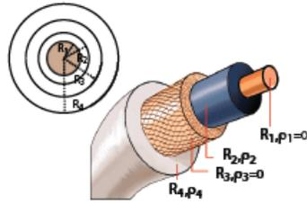
Figura 4: Cable coaxial infinito
