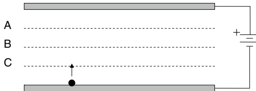
FIGURE 7.6 Parallel plates 8 cm apart and a 5 nC charged particle in an electric field of E = 2.5 \times 10^4 \text{ N C}^{-1} (see Problem 6).
