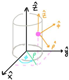
$$\begin{aligned}\vec{r} &= \rho\hat{\rho} + z\hat{z} \\ \vec{v} &= \dot{\rho}\hat{\rho} + \rho\dot{\phi}\hat{\phi} + \dot{z}\hat{z} \\ \vec{a} &= (\ddot{\rho} - \rho\dot{\phi}^2)\hat{\rho} + (2\dot{\rho}\dot{\phi} + \rho\ddot{\phi})\hat{\phi} + \ddot{z}\hat{z}\end{aligned}$$
