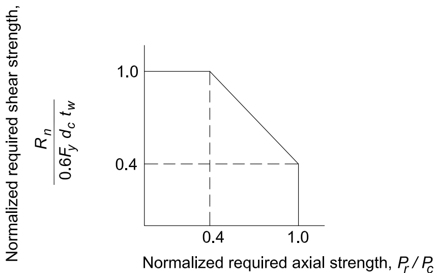
Fig. C-J10.4. Interaction of shear and axial force—elastic.
