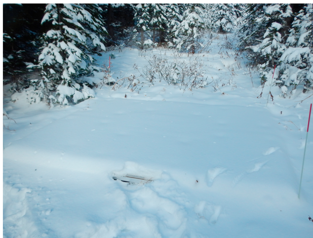
Figure 14. Load cell measurement device with rectangular plates buried under a layer of snow. This sensor was installed at a field site in the Rocky Mountains of Canada. Some uneven settling of snow is present around the load cell device.
