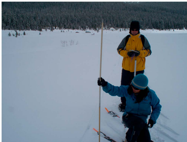
Figure 1. Snow depth rod measurement of snow depth. The investigator in the background is recording a measurement of snow depth read by the observer in the foreground.
