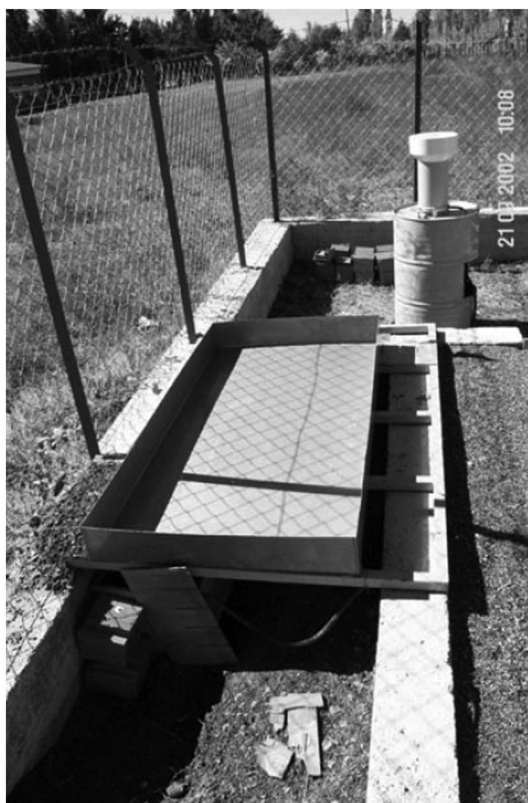
Figure 17. Picture of snowmelt lysimeter installation at Guzelyayla Station in Turkey [from Tekeli et al. , 2003]. Further details on the design of the system are given by Tekeli et al. [2003].
