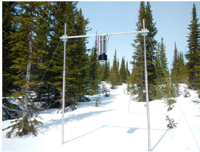
Figure 27. Photograph of GMON installed at a field site in the Rocky Mountains.
