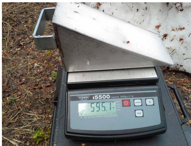
Figure 8. Photograph of a triangular sampler being used with a scale to determine the mass of snow within the sampler.
