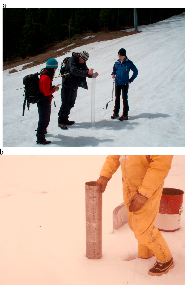
Figure 4. (a) Snow tube sampling on a slope using a plastic-body ESC30 snow tube. After a snow sample is extracted, the ESC30 is weighed on a spring scale. (b) Container with 6 inch diameter (15.3 cm) used as gravimetric snow tube sampler [from Dyck, 1969].
