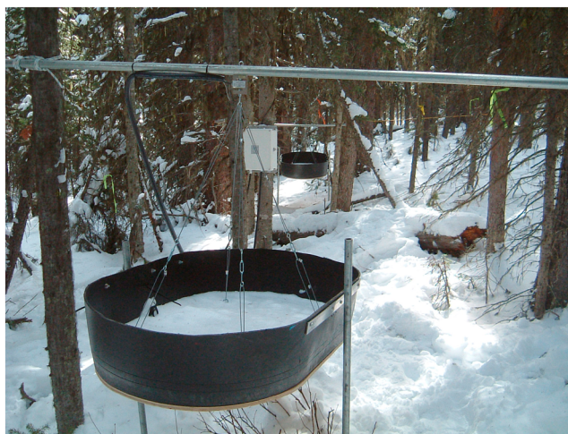
Figure 15. Hanging lysimeter used to measure unloading of intercepted snow from a forest canopy at the Marmot Creek Research Basin.
