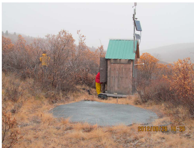
Figure 13. Classical snow pillow installation on the ground surface at a field site in northern Canada. Snow accumulates on top of this pressure transducer over the winter season. Visible in the background is a small control shed with the manometer and associated apparatus.
