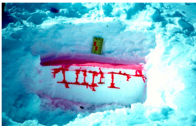
Figure 7. A dye tracer experiment being used to visualize meltwater flow paths in a snowpack (photograph courtesy of Dr. Phil Marsh).
