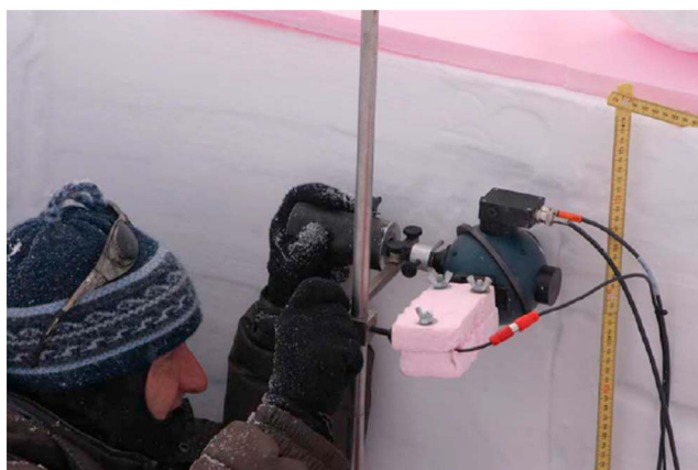
Figure 22. Measurement of SSA using an integrating sphere [from Montpetit et al. , 2011].
