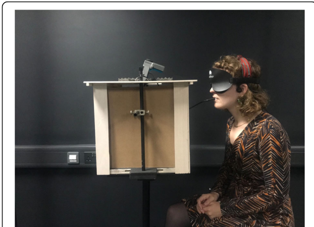
Fig. 3 Image showing a user wearing an auditory-tactile cross-modal display prototype. The tactile information is created by BrainPort, a visual-to-tactile sensory substitution device. The auditory information is created by The vOICE, an auditory-to-tactile sensory substitution device. The camera fixated within the box provides real time feed to BrainPort and The vOICE. As a result, the user can perceive the camera feed via audio, tactile and audio-tactile cross-modal feedback
